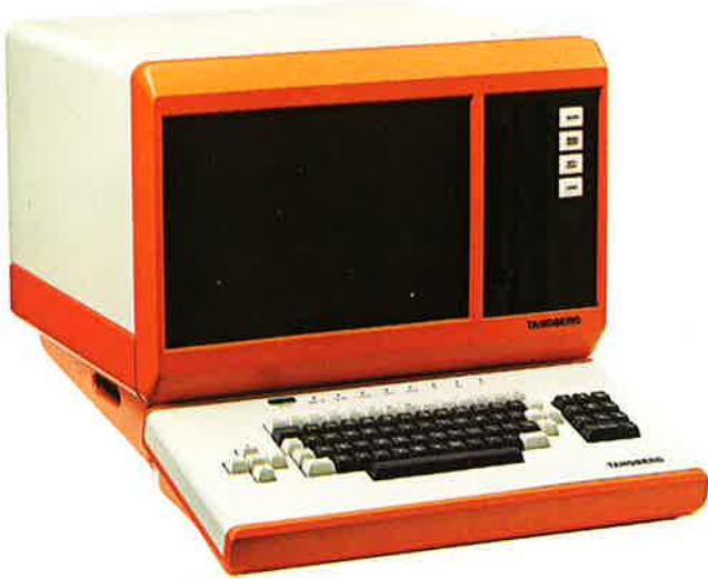
TDV 2114 with built-in diskette drive or cartridge recorder. The diskette with particular advantage in fast access of data and the cartridge with large storage capacity.
