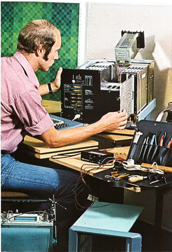
The terminal is designed with easy and fast servicing in mind. The modular construction enables the service engineer to easily substitute modules, causing a very short Mean Time To Repair (MTTR).
