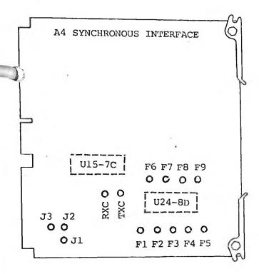
The signal Output Interrupt Enable (OIE) is connected to a pull-up resistor through the printed circuit. Provisions are however made so that OIE may be generated by a flip-flop. Such a version of the Synchronous Interface will be equipped with a jumper in position J1 to J2.
