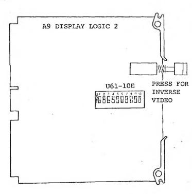
The INVERSE VIDEO push switch is located to the right of switch U61.
