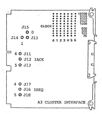
The setting of the jumpers on the Cluster Interface depends on whether the system consists of one or two Cluster Interface boards.
