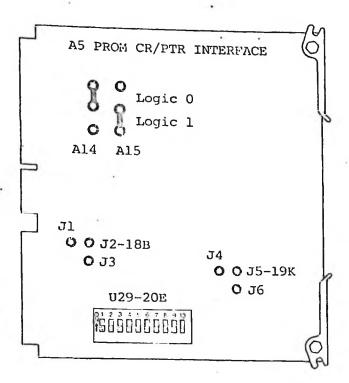
The Memory Allocation Switch consists of two jumpers that can be positioned four different ways to obtain the desired memory allocation. See table below:
