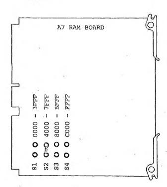
The Memory Allocation Switch can be set in one of four possible positions.
