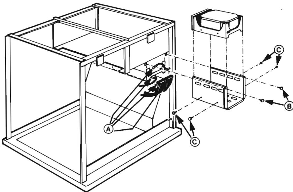
Figure 36. Replacing a Disk Drive
