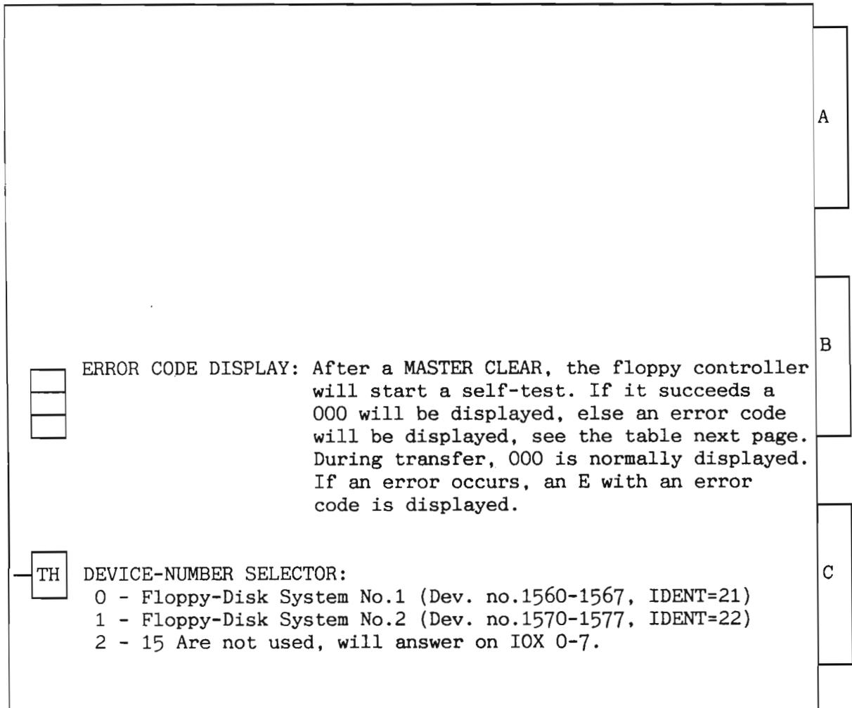
*Figure 57. Floppy Disk Controller for DMA (3027)*
