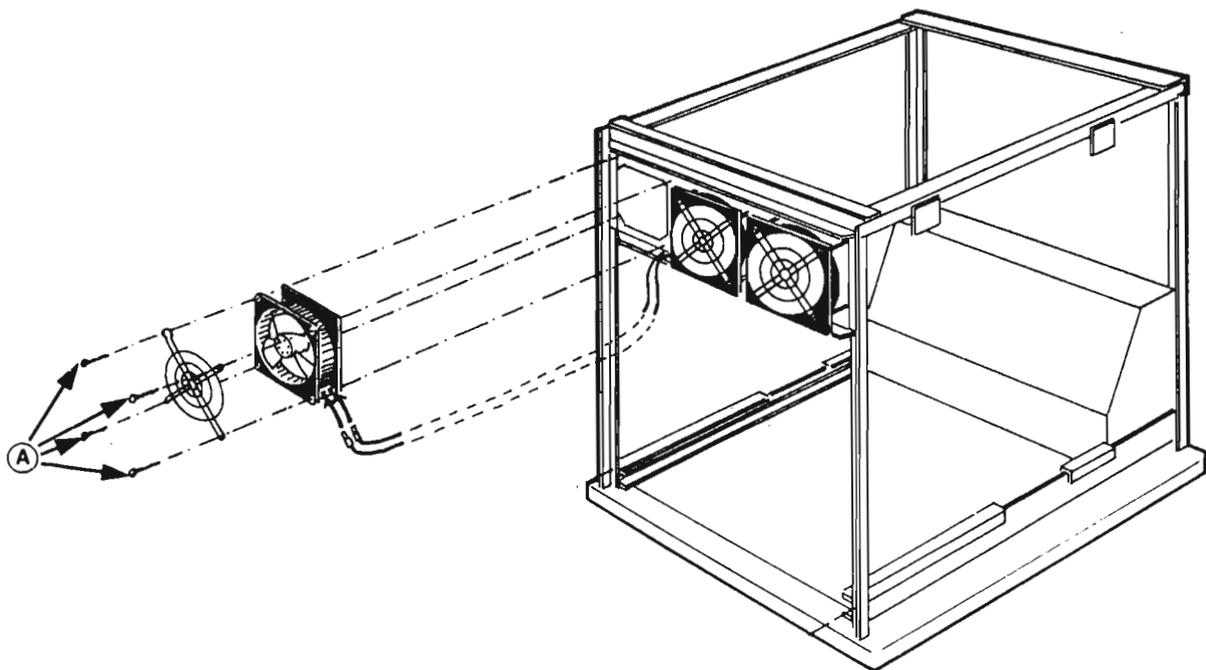
*Figure 37. Removing a Fan (I)*
