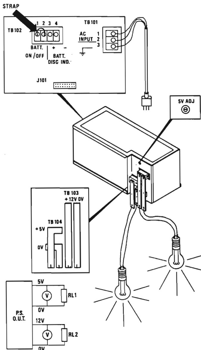
Figure 22. Approximate Adjustment of the Standby Power Supply
