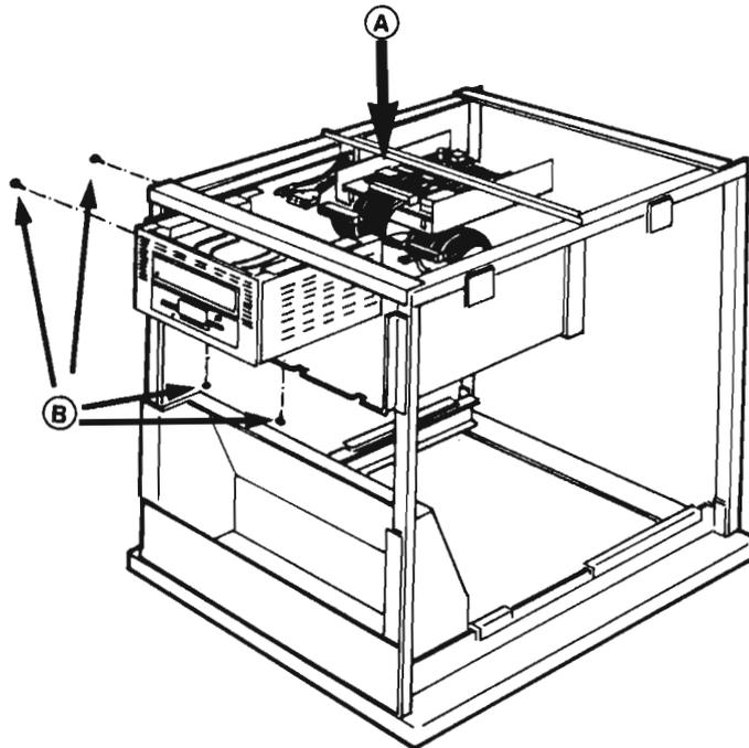
Figure 32. Replacing a Floppy Drive (I)
