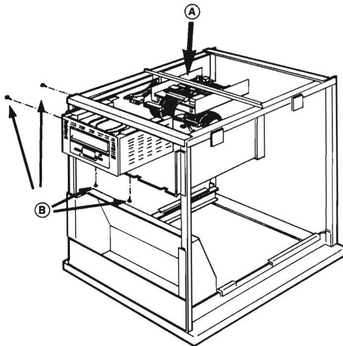
Figure 34. Replacing a Streamer (I)
