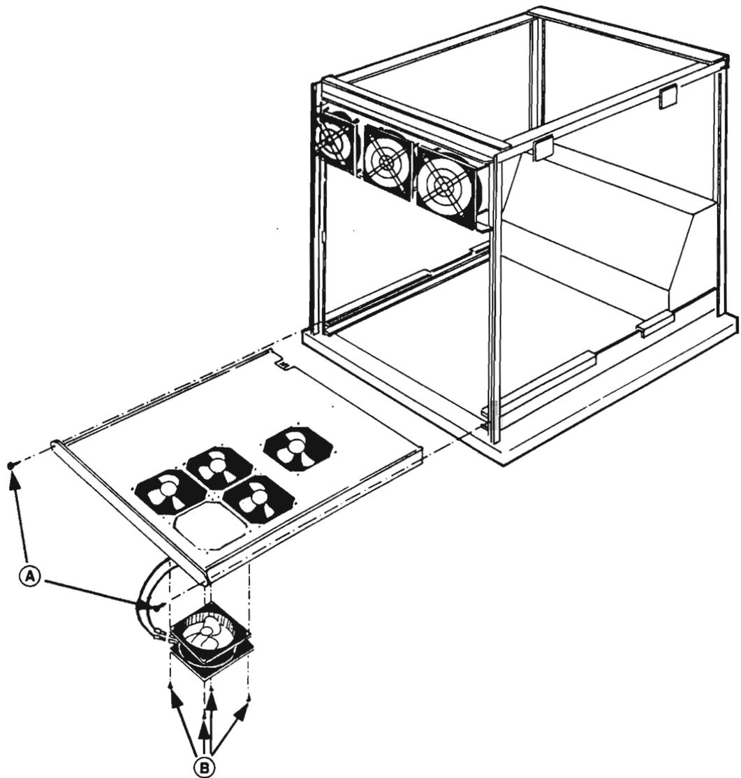
Figure 38. Removing a Fan (II)
