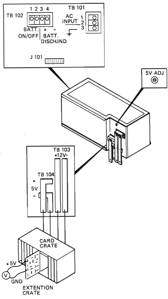
Figure 23. Fine Adjustment of the Standby Power Supply
