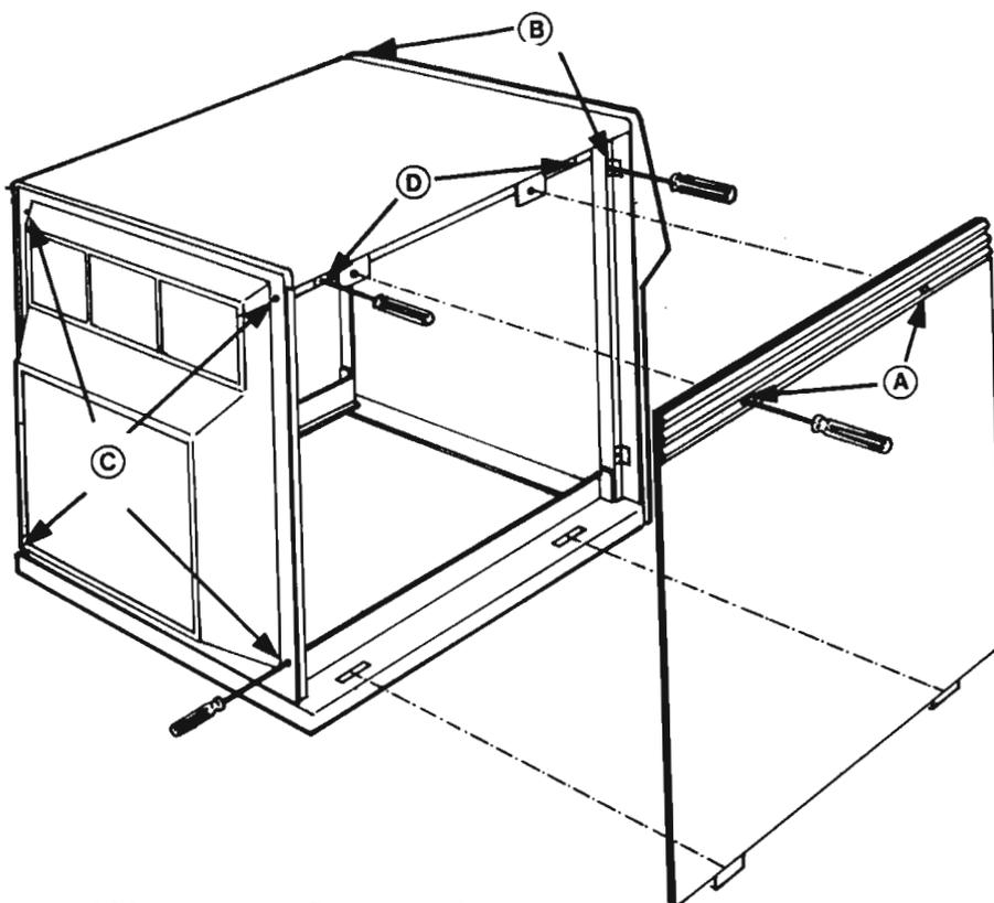
Figure 30. Removing the ND-100 Compact Cabinet Panels
