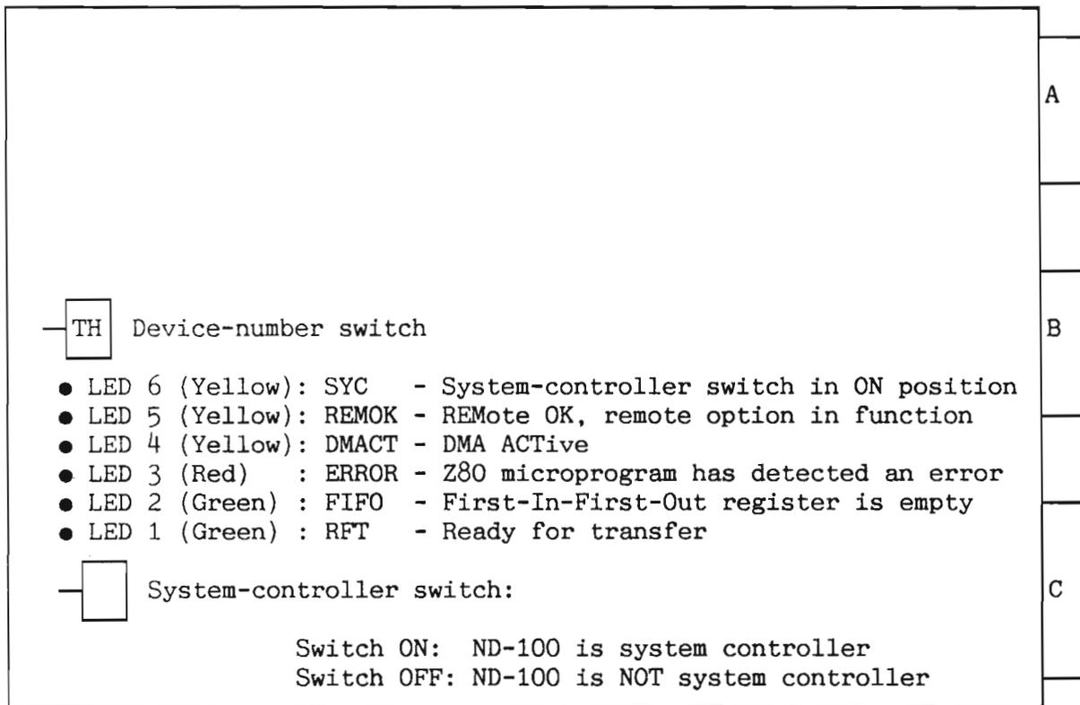
Figure 56. GPIB Controller (3026)
