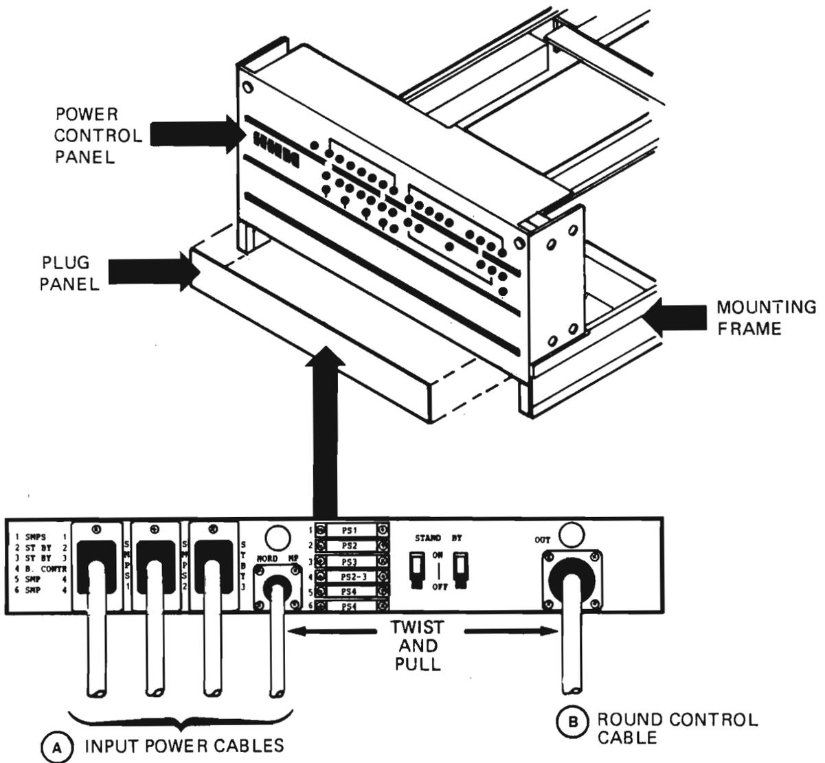
Figure 17. Input Power Cables
