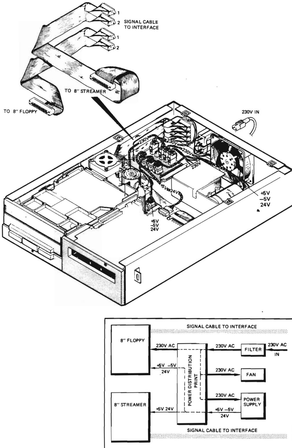
Figure 8. AC and DC Distribution for Floppy and Streamer Drive
