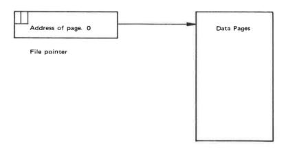
An index-sequential file is defined by a 1K index block, which contains pointers to the 1K data pages of the file:
