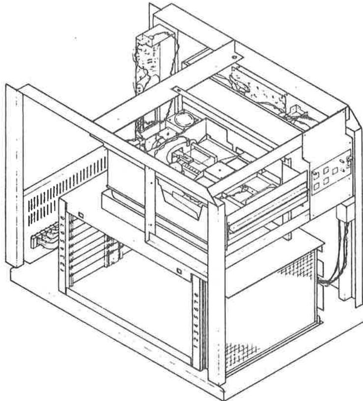
Fig. 9. Cabinet Layout showing Card Rack on left
