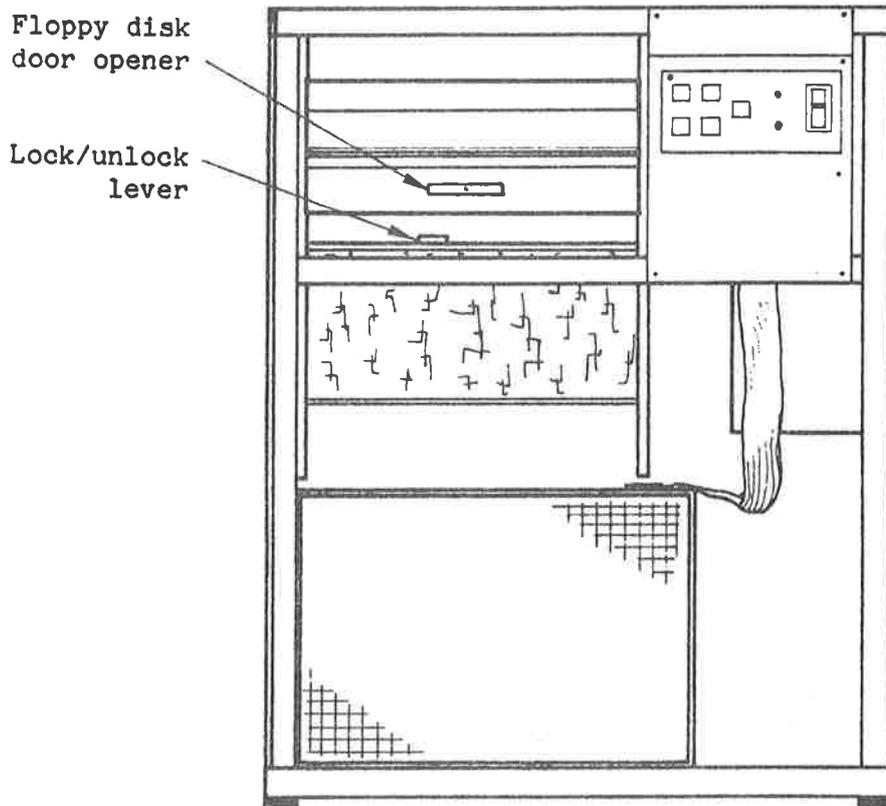
Fig. 5. Satellite front view with front cover removed
