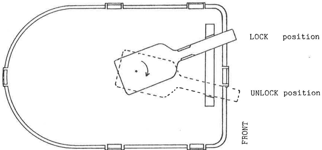
Fig. 6. Top view of disk drive with lock/unlock lever
