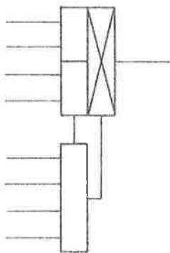
The four-input gates are 7460 circuits
