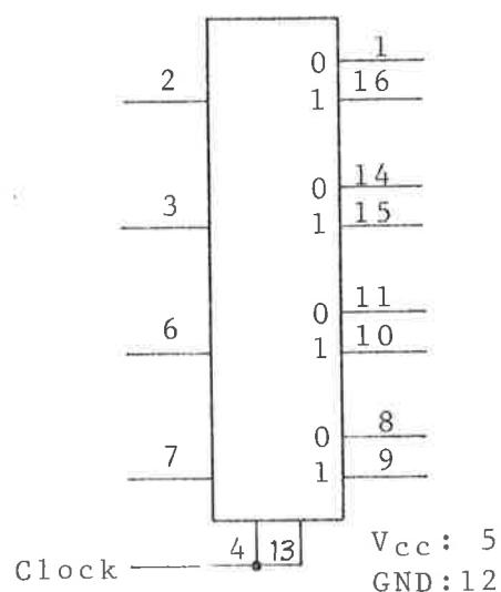
The clock input on pins 4 and 13
