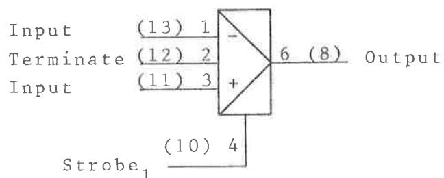
Pins 1 and 2 (13 and 12) are connected when internal termination resistor is used.
