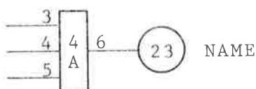
Input terminals are if possible to the left and output to the right. The distance between input lines should be 5 mm. If an unused input terminal is connected to a used terminal this should be shown in the diagram. Circled numbers represent card terminals.
