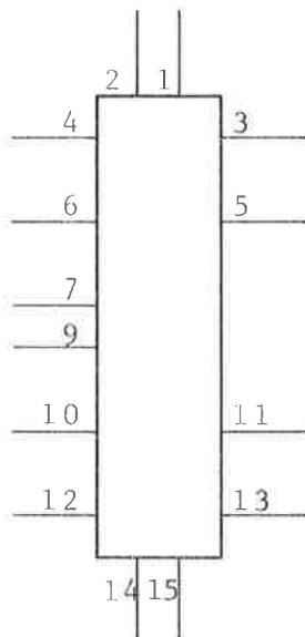
Pins 7 and 9 connected to GND
