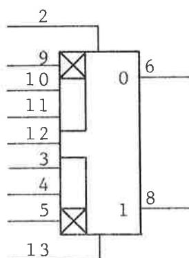
The AND gate opposite the 0 output is equal to K-inputs.
