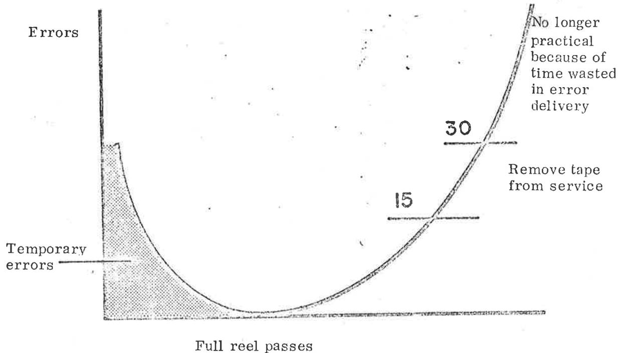
A new reel of tape will exhibit a number of temporary read errors when first used.
