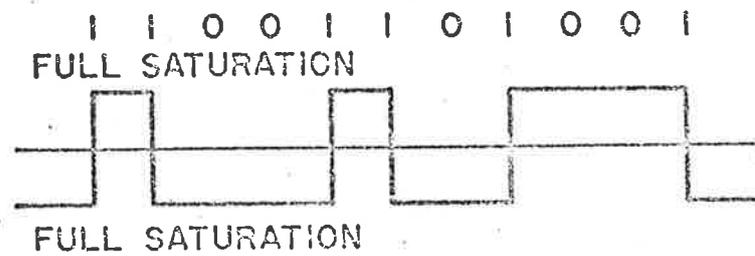
NRZI means non return to zero invert. This method inverts (reverses) the direction of magnetic flux on tape each time a logical one is written.
