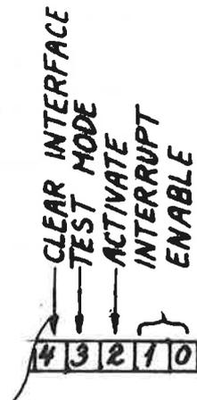
The transfer is initiated by setting the CONTROL-WORD REGISTER informing of:
