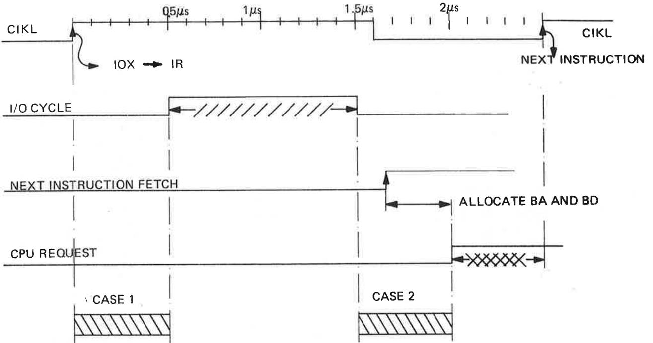
////// The Main and Local I/O bus is used by the IOX instruction. The CPU data bus IB is also allocated for the IOX instruction.
