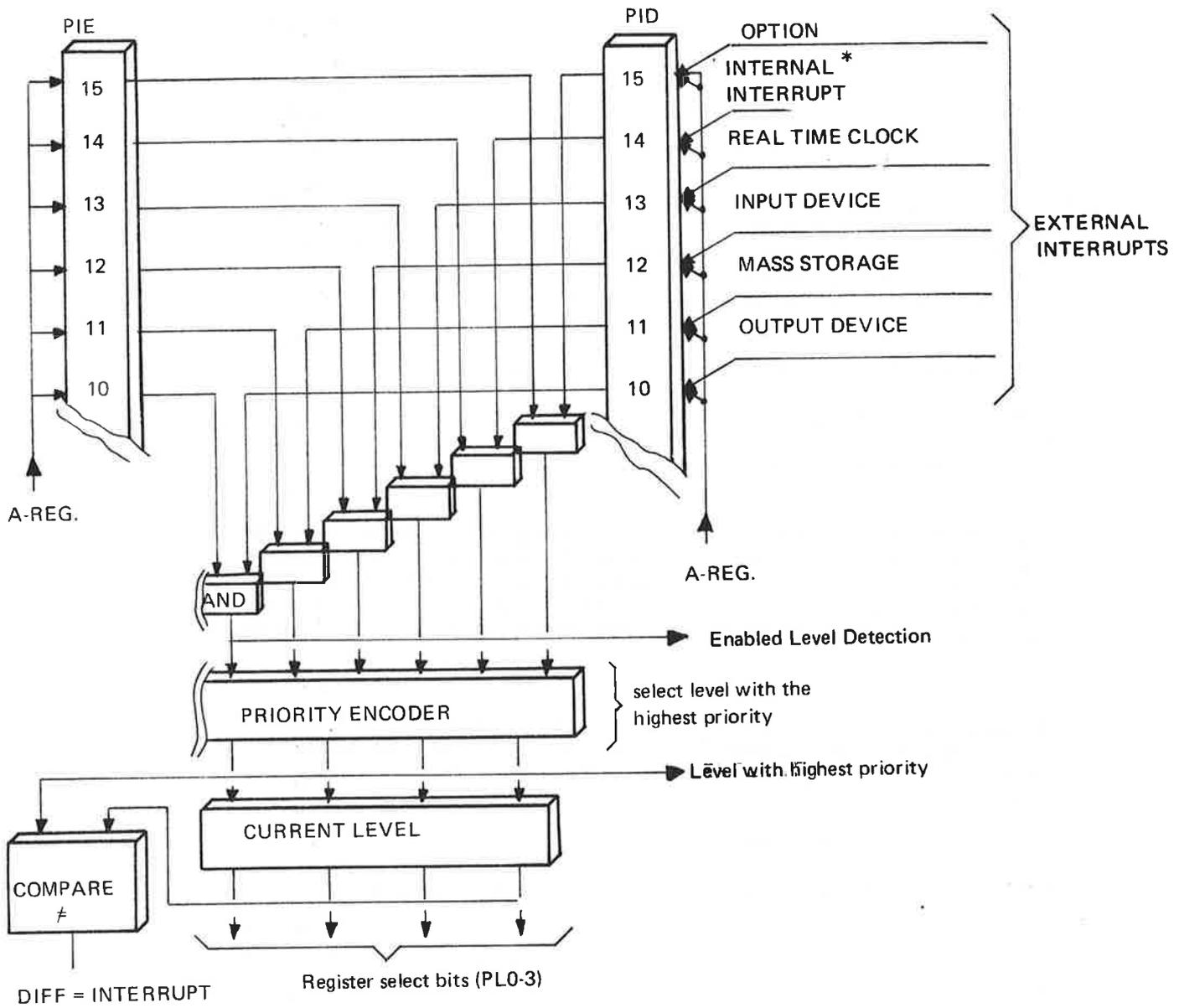
\* Internal interrupt LEVEL 14 NO CONNECT error, IOX-timeout is one source.
