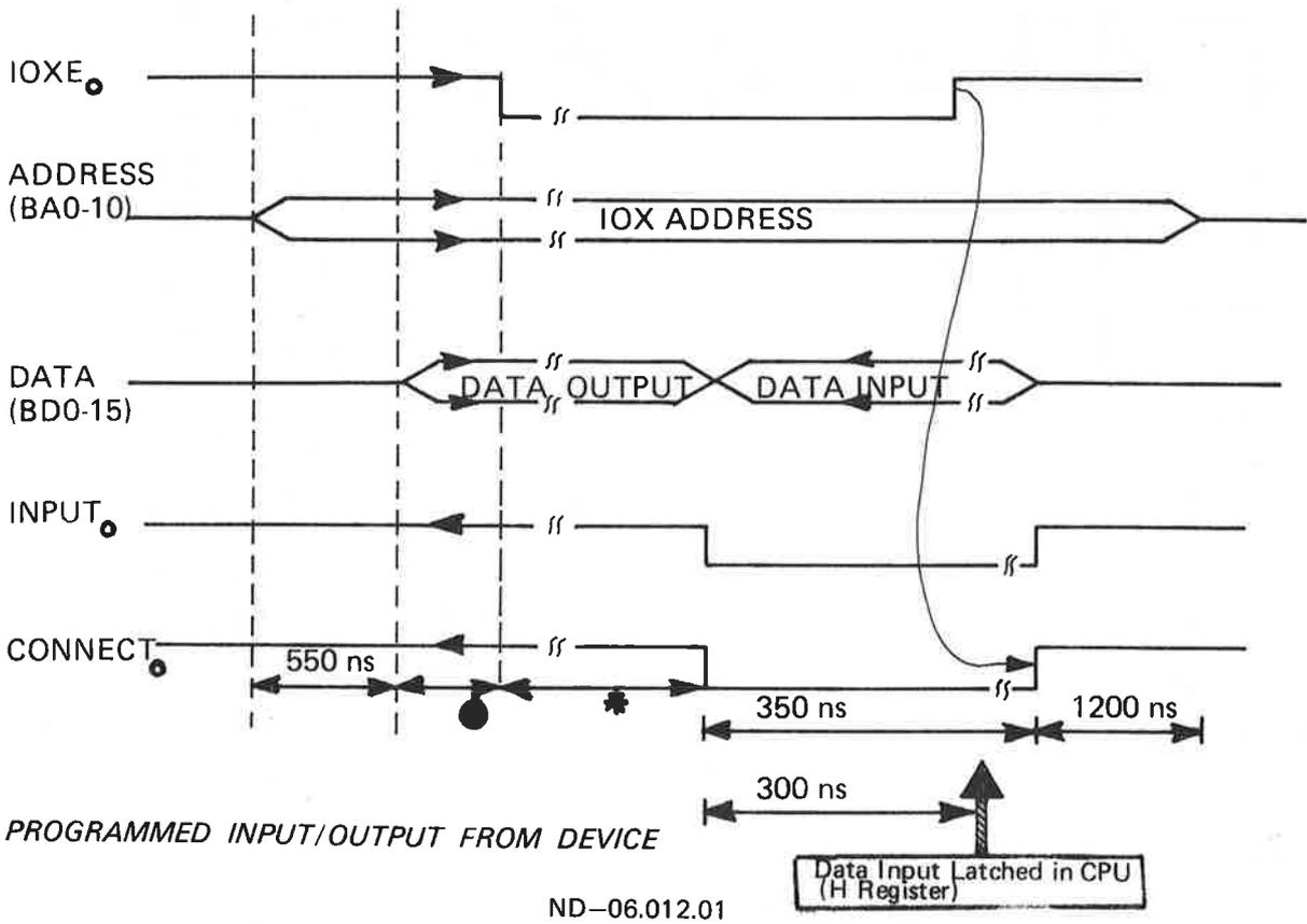
Figure 2.3: PROGRAMMED INPUT/OUTPUT FROM DEVICE
