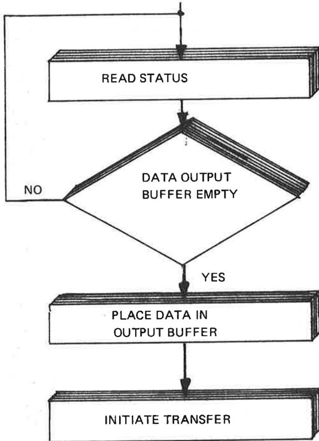
The interface STATUS-REGISTER is read, and bit 3 is checked for a 1. If a 1, this implies that the previous data transfer was finished and new data can be placed in the output data buffer. If NOT, loop.
