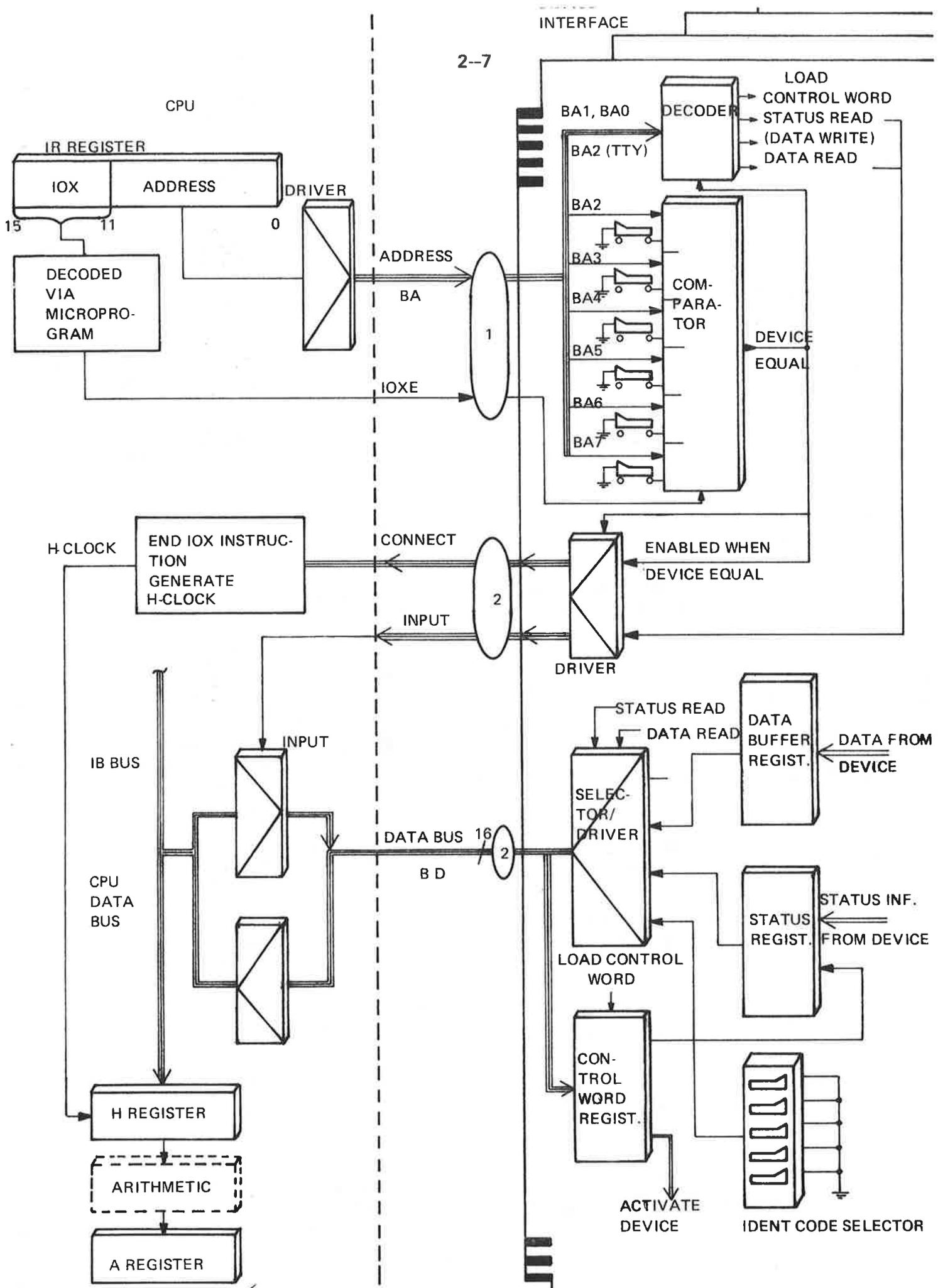
Figure 2.2: NORD-10/S COMMUNICATION WITH PIO INPUT INTERFACE
